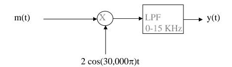
The output y(t) is the scrambled version of the input signal m(t). Let the spectrum of the signal m(t) be as shown below, write m(t) as a function of y(t)
