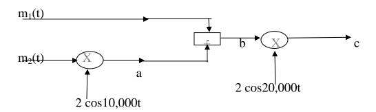
The modulated signal at point c is transmitted over a channel. Determine the bandwidth of the output signal at point c.
