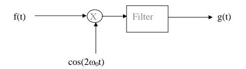
The filter in the above figure is considered to be a unity gain ideal band-pass filter of mid-frequency ( $\omega_0$ ) and bandwidth (2W) rad/s. Determine the output of this filter. Assume that rect(t/T) has a bandwidth of W rad/s.
