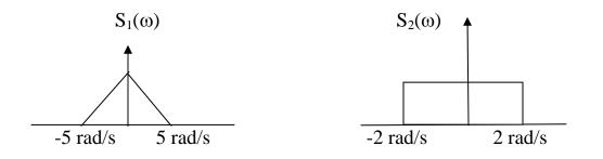
Determine the bandwidth of the signal y(t) given by:  $y(t)=s_1(t)+10s_2(t)\cos 10t$ .
